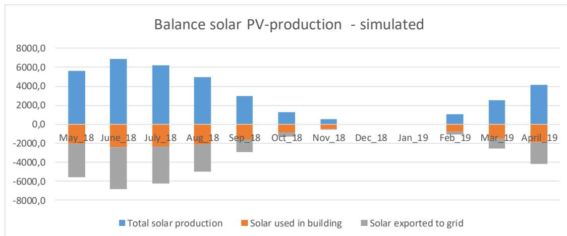
**Figure 5. The simulated solar PV production and split between use in building and exported to the grid.**
