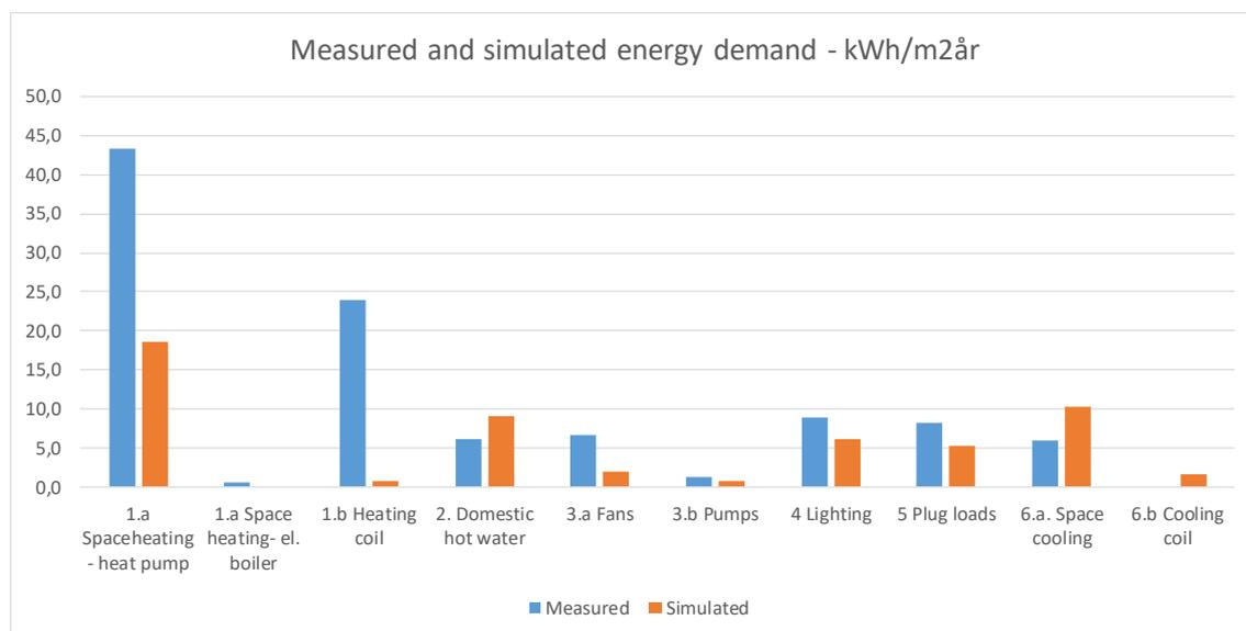
**Figure 6. Measured and simulated net energy demand.**
