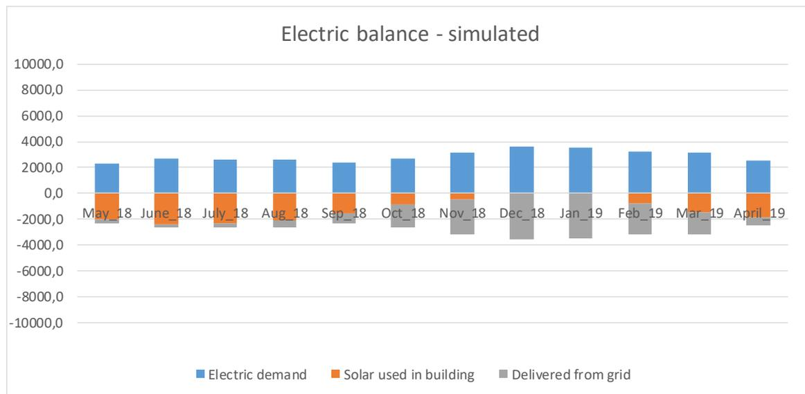
**Figure 3. The simulated monthly electric balance of the building.**
