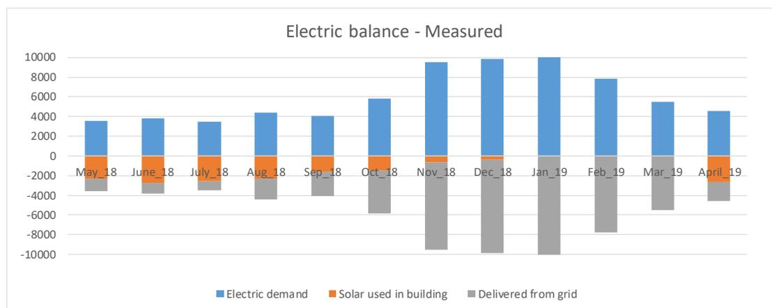
**Figure 2. The measured monthly electric balance of the building.**
