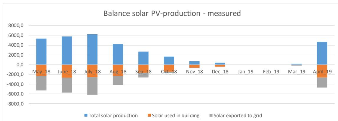
**Figure 4. The measured solar PV production and split between use in building and exported to the grid.**
