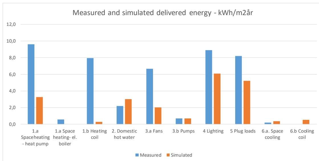
**Figure 7. Measured and simulated net energy demand.**
